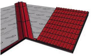
Lay the full-size roofing panels. Leave the panels that require cutting uninstalled at this stage.
