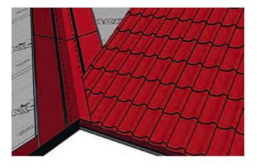
Install the cut panels up to the top of the valley, making sure as you proceed that the angle of the valley follows the guide line you have drawn.
