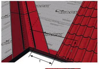
Measure the space for the panel, measuring from the guide line to where the panel overlap ends.
